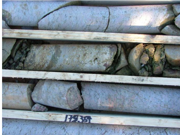
Figure 3. Weathered gneiss at 173 meter in KB5336.
